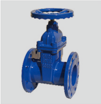
BS5163 Resilient Seated Gate Valve Type: NRS,Flange End Size:DN40-DN1200 Class:PN10,PN16,PN25
