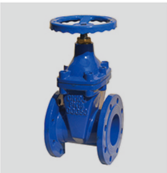
DIN3352 F4 Heavy Type Resilient Seated Gate Valve Type: NRS,Flange End Size:DN50-DN1200 Class:PN10,PN16,PN25
